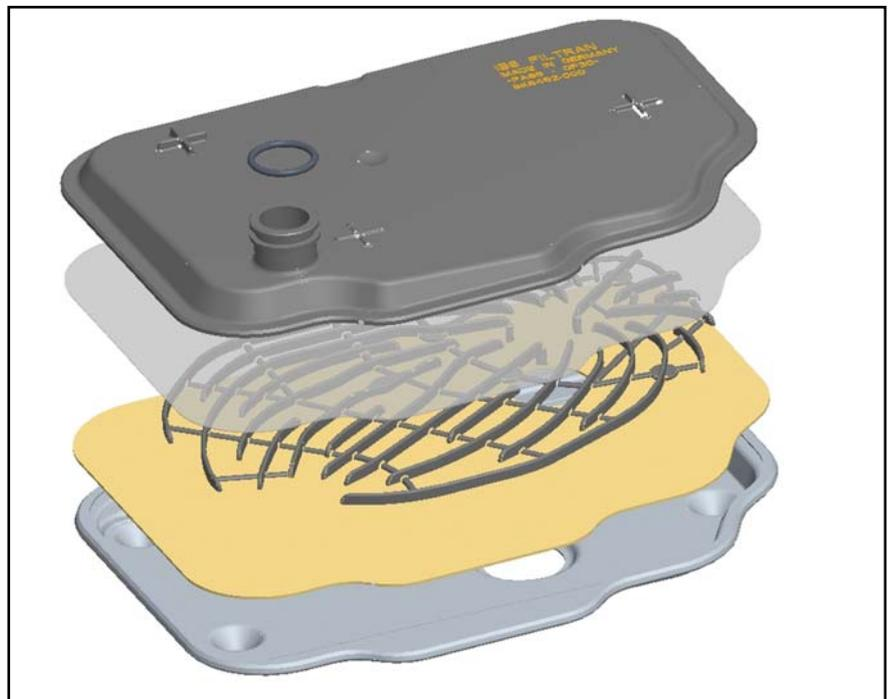
Figure 1: Structure of a CombiMedia™ suction filter from top to bottom: filter housing upper cover, full-flow screen mesh, rib tray as spacer, partial-flow fine filter medium, and filter housing bottom pan
