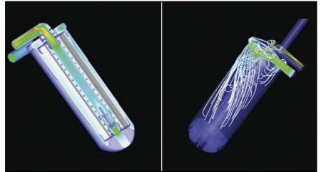
Figure 2: View of the velocity distribution (left) and streamlines (right) inside a pressure filter
