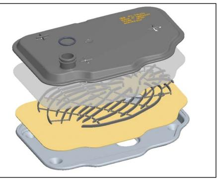
Figure 1: Structure of a CombiMedia<sup>™</sup> suction filter from top to bottom: filter housing upper cover, full-flow screen mesh, rib tray as spacer, partial-flow fine filter medium, and filter housing bottom pan
